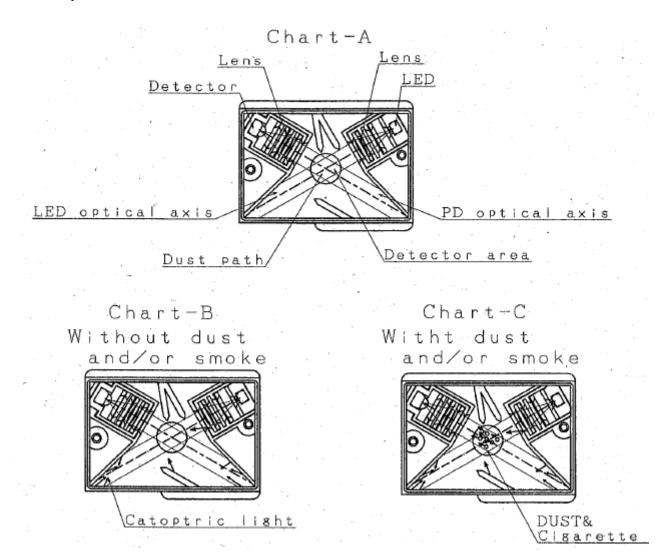
Light from the light emitter (Light Emitting Diode) is spotted with a lens and a slit as shown on the chart-A. Also for the light detector (Photodiode), a lens and a slit is positioned in front of it to cut disturbance light and to detect light reflection (when detecting dust) efficiently. Area where those two optical axis cross is detection area of the device.
