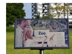
Reflective IGZO display with high outdoor visibility
