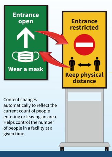
A sensor installed on a display stand counts the number of people entering or leaving a facility. That information is then used to automatically switch preset content (A or B) depending on the number of people entering or leaving.
